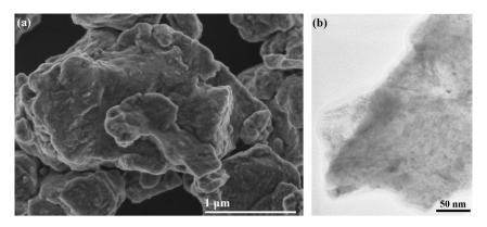
Fig. 2. Electron micrographs of Al/ZrSiO<sub>4</sub>/B<sub>2</sub>O<sub>3</sub>/C system after 3 h milling, (a) SEM and (b) TEM images.
