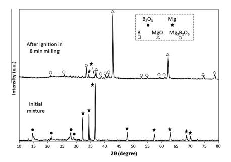
Fig. 7. X-ray diffraction patterns of initial and milled samples of Mg/B<sub>2</sub>O<sub>3</sub> system.
