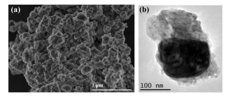
Fig. 9. Electron micrographs of Mg/ZrSiO<sub>4</sub>/B<sub>2</sub>O<sub>3</sub>/C system after 3 h milling, (a) SEM and (b) TEM images.
