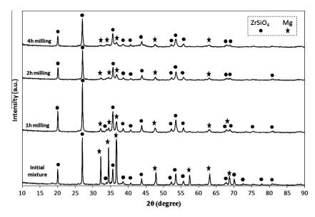
Fig. 8. X-ray diffraction patterns of initial and milled samples of Mg/ZrSiO<sub>4</sub> system.
