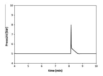
Fig. 6. Pressure inside the vial versus milling time for Mg/B<sub>2</sub>O<sub>3</sub> system.
