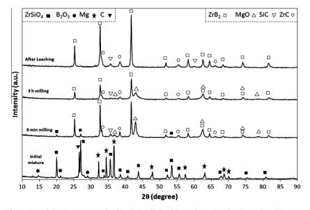
Fig. 4. X-ray diffraction patterns of as-blended, milled and leached samples of Mg/ZrSiO<sub>4</sub>/B<sub>2</sub>O<sub>3</sub>/C system.
