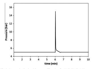
Fig. 3. Pressure inside the vial versus milling time for Mg/ZrSiO<sub>4</sub>/B<sub>2</sub>O<sub>3</sub>/C system.
