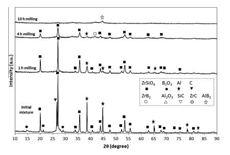
Fig. 1. X-ray diffraction patterns of as-blended and milled samples of Al/ZrSiO<sub>4</sub>/B<sub>2</sub>O<sub>3</sub>/C system.
